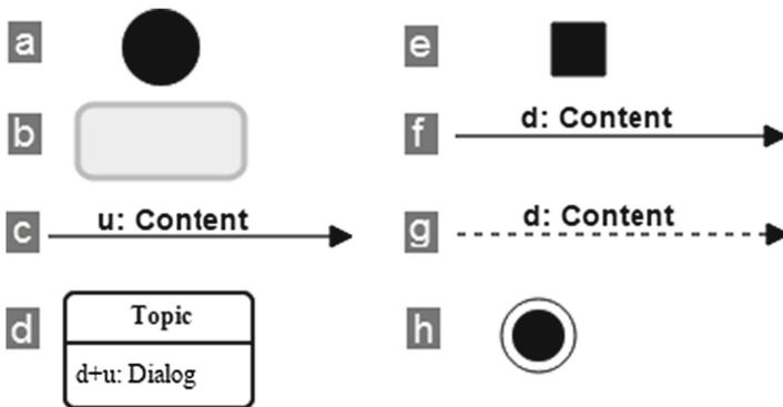
**Fig. 2.** Elements of the MoLIC language, where: **a** is the opening point; **b** is a ubiquitous access; **c** is a user utterance; **d** is a conversation scene; **e** is a system processing; **f** is a designer utterance; **g** is a breakdown utterance; and **h** is a closing point.
